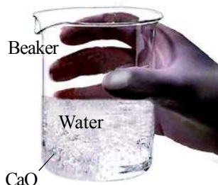
fig-7: Formation of slaked lime by the reaction of CaO with water
