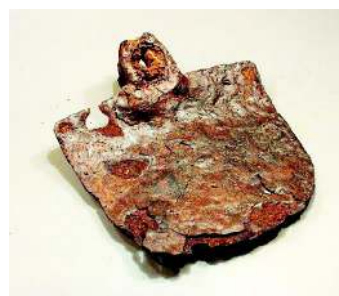
fig-17: Rusting of iron
